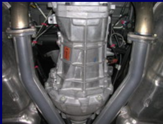
You can see the electrical plugs I installed tied up with red tie-wraps waiting for the cutouts.
