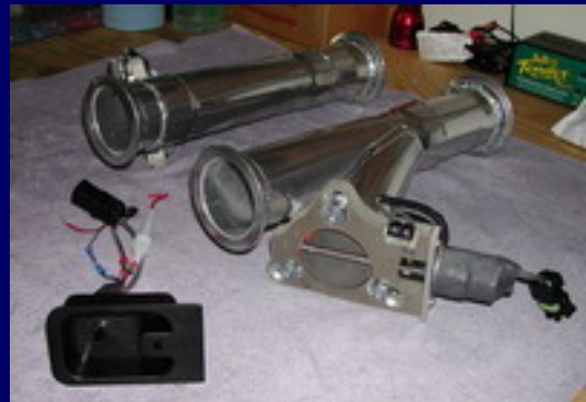
The FLP cutouts with McCord electrics and the switchbox. I was hoping these was going to just fit in place of the existing FLP cats. They were too wide to fit . Time for 'Plan B'.
