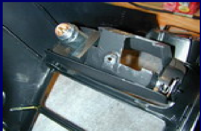
Clearance for the switch cut out of the IP trim panel
