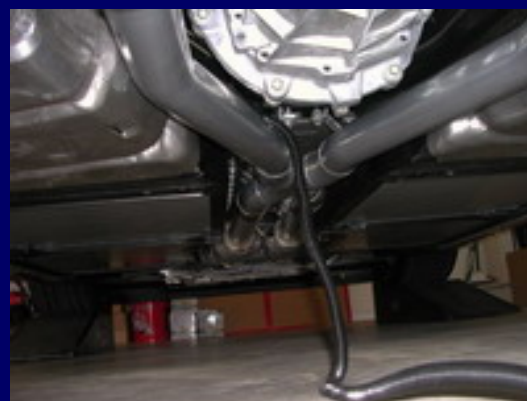
Attached the cable to fish tape with duct tape and pulled it through to the cabin
