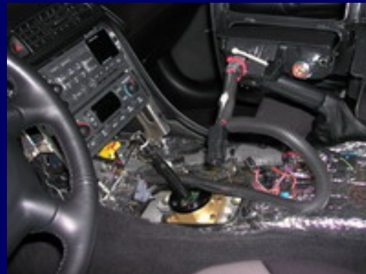
Wire loom added to protect the wiring
