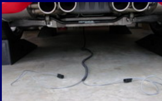
Laid the cabling out in preparation for the pull up the torque tube tunnel
