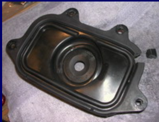
Clearance-notched the shifter isolator for the wiring
